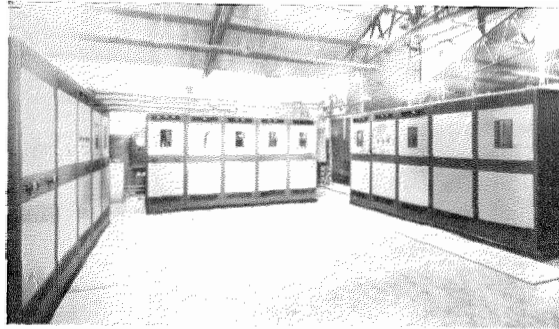
Fig. 22—40 kW (peak) Ultra-Short Wave Transmitter for Television.
